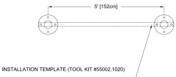
REFER TO MAINTENANCE MANUAL FOR INSTRUCTIONS ON INSTALLATION DETAIL AND TOOL KIT #55002.1020 MUST BE USED DURING CONCRETE POURING FOR THE PLACEMENT OF THE SAFESWAP TO ENSURE CORRECT PLACEMENT FOR FEATURES.
